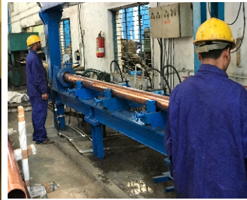
Hydrostatic Pressure Test
